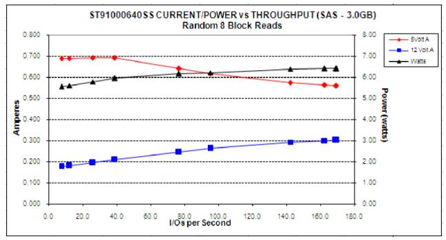
Figure 3. 1TB Models (3Gb) DC current and power vs. input/output operations per second
